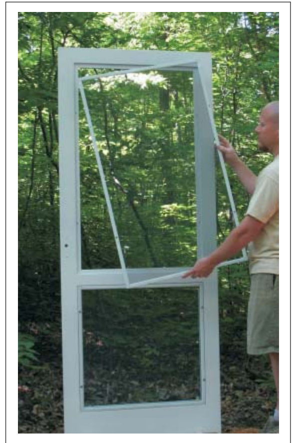
Two removable panels sit in a rabbet, flush with the inside of the door, dividing at the middle rail. They are easily removed with a flat head screwdriver. The aluminum screen and storm frames are available in white or dark bronze.
